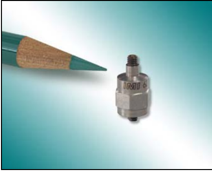
Figure 5: The Model 621B40 high frequency accelerometer from IMI Sensors operates to 30k Hz, even with a magnet. Because of its wide frequency range, the sensor can be used to diagnose a variety of machinery fault conditions, including bearing and gear problems.
